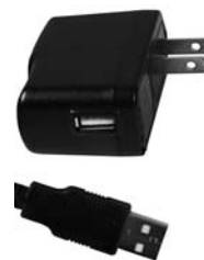
optional USB-type external power supply
